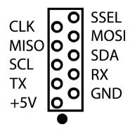
This connector allows use of EX, I2C and UART protocol devices.
