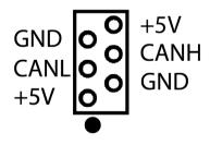
This connector allows use of CAN protocol devices. **PLEASE NOTE:** CAN INTERFACE IS CURRENTLY UNDER DEVELOPMENT
