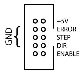
Each connector controls one motor driver. Controller has 4 connectors for axes 1-4. Pins 2, 4, 6,7, 8 and 10 provide the 'Ground' or common side of connections.
