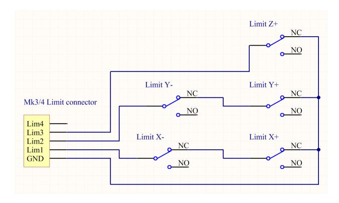
Serial wiring of NC type limit switches\*:
