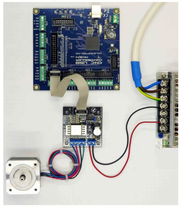
Picture bellow demonstrates connection of motor driver to Mk3/4 controller and connection of controllers external power supply:
