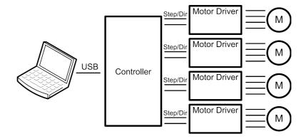
The PlanetCNC series of USB CNC motion controllers is link between a personal computer and motor drivers supporting step/direction control. PlanetCNC series of motion controllers are compatible with most motor drivers. The controllers use the USB port, available on all modern computers and laptops. They can serve as direct replacement or upgrade for many parallel port break-out boards.
