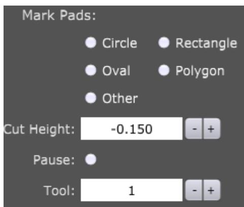
You can mark selected pad shapes to ease manual drilling later. Software will recognize shapes: Circle, Oval, Rectangle, Polygon or Other(custom).
