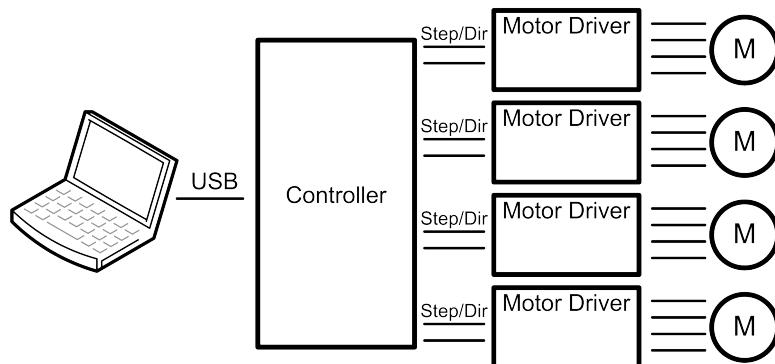
The PlanetCNC series of CNC motion controllers are link between a personal computer and motor drivers supporting step/direction control. They are compatible with most drivers. The controllers use the USB or Ethernet port, available on all modern computers and laptops. They can serve as direct replacement or upgrade for many parallel port break-out boards.
