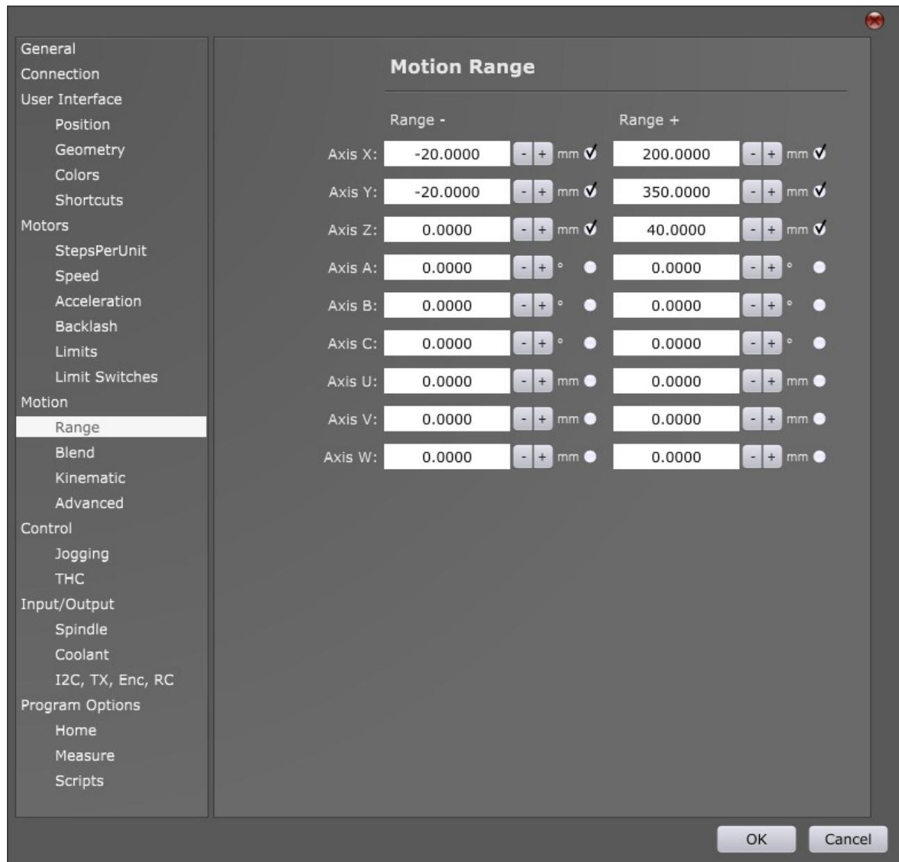
When you set and enable your machines motion range values, you will notice that 3D representation of motion range limits will be displayed accordingly on the main screen:
