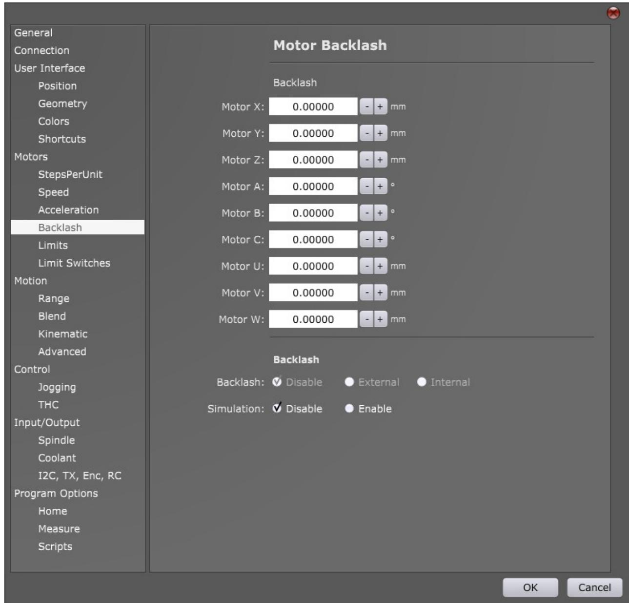
Units of backlash compensation values for linear axes are in mm, for rotational axes are in degrees.
