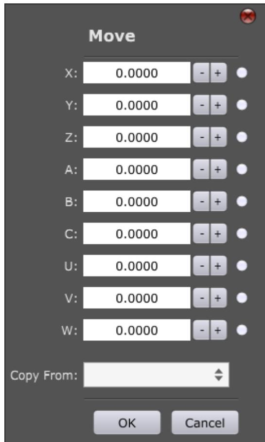
You can move all 9 axes: **X,Y,Z,A,B,C,U,V,W**. To move selected axis to specified position, enable axis radio button, insert axis position and click OK.
