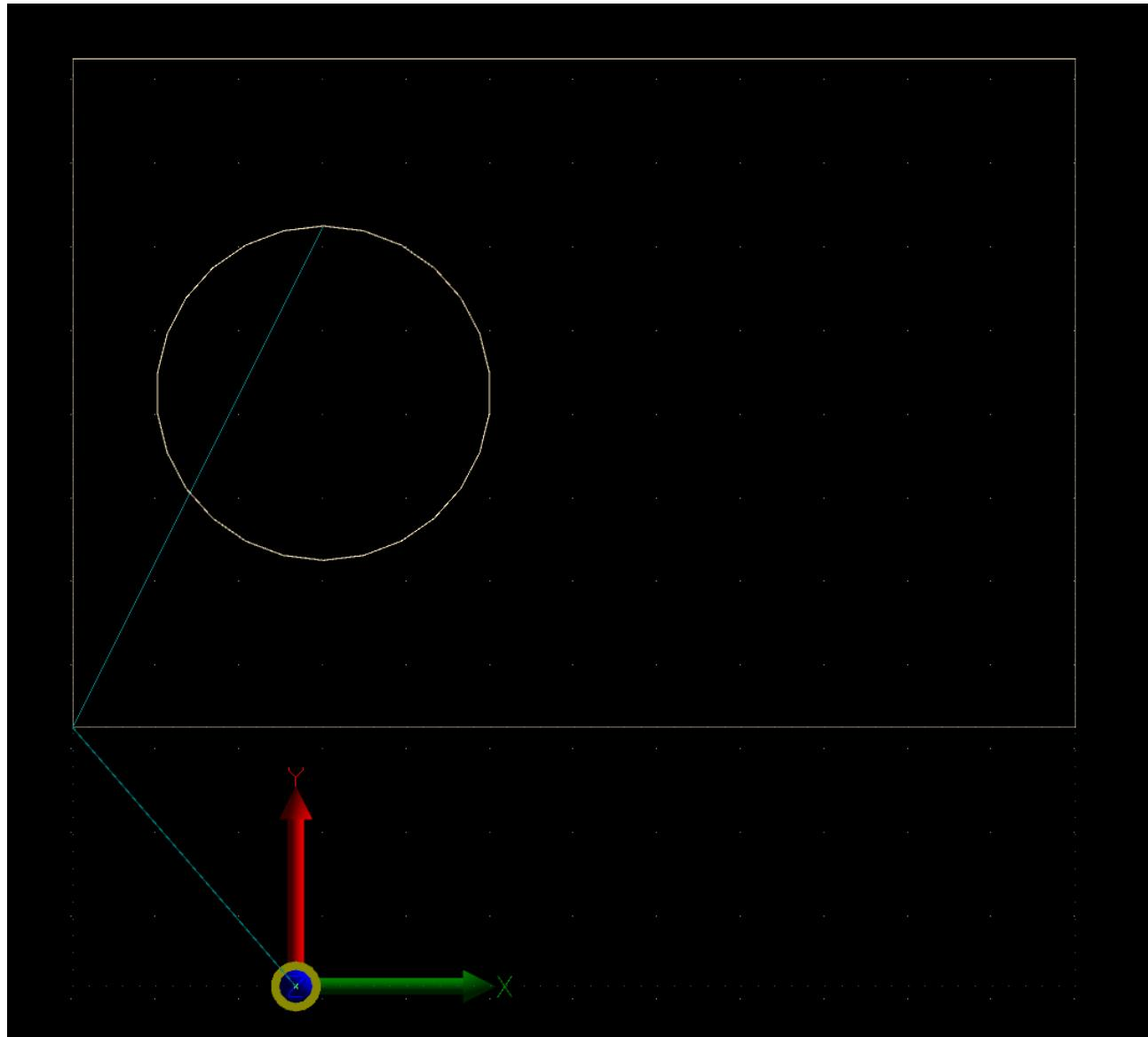
Generated toolpath is positioned in relation to its absolute XY 0,0 coordinates (the way it was drawn). But what if we want that toolpath extents are aligned with working position XY0,0?
