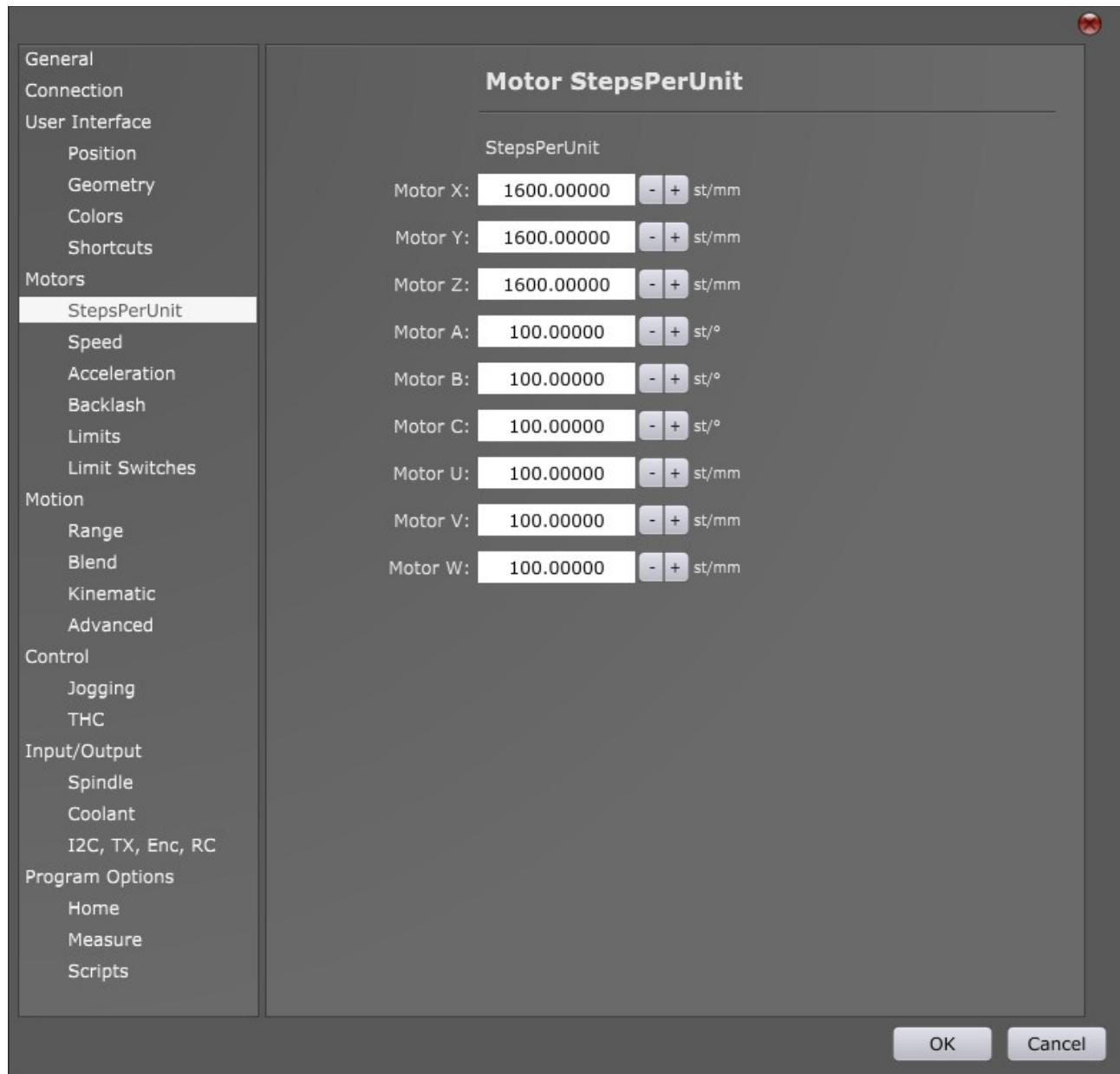
Motor settings for linear axes X,Y,Z, U ,V, W use steps per millimeter units (st/mm) while motor settings for rotational axes A, B, C use steps per degree units (st/°).
