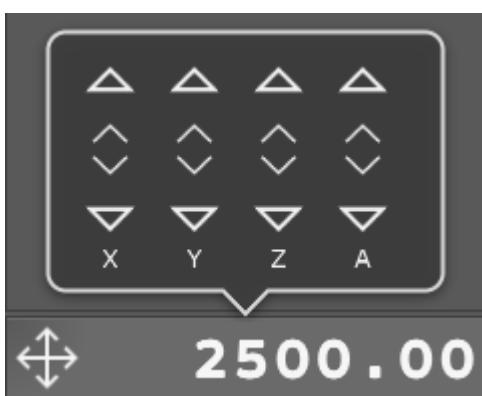
Mouse click+hold on large arrow jog buttons to jog machine in desired direction. Machine will move until the mouse button is released. Corner buttons allow diagonal or combined axis jogging.
