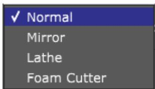
Each preset automatically adjusts *Rotate&Mirror*, *Axis* and *Orientation* parameters so that 3D axis and tool display suit to corresponded machine type(E.g.: Lathe and Foam Cutter).
