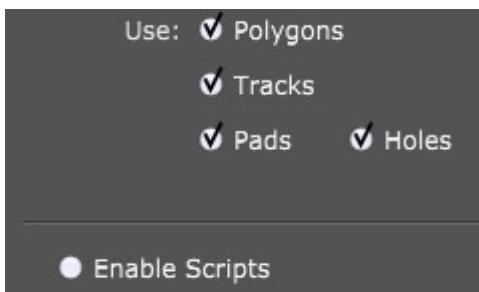
Gerber files can contain different elements such as polygons, tracks, pads and holes.
