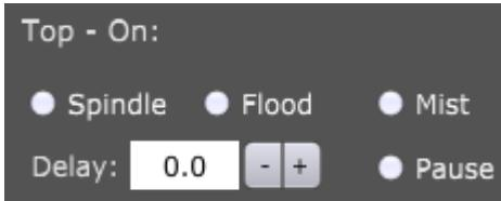
Inserts ON g-codes for Spindle, Flood, Mist (M3,M7,M8), Delay and Pause before cut, before moving down from Safe Height to cut (or pass) height.
