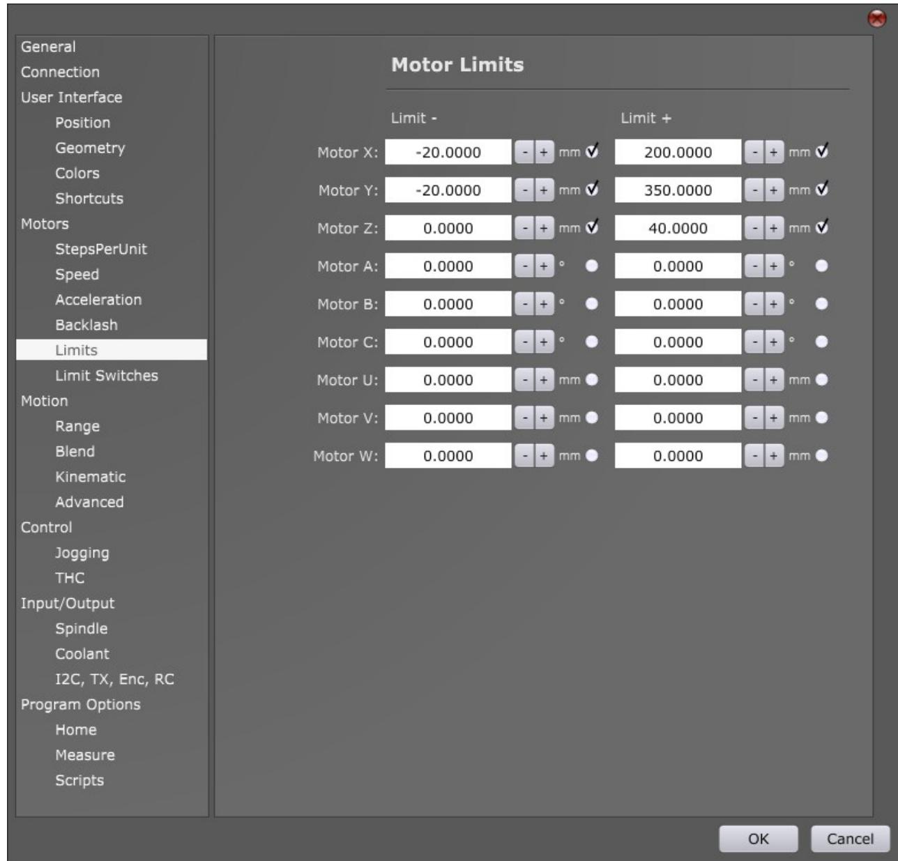
**Limit-** value sets limitation of motor movement in negative direction.
