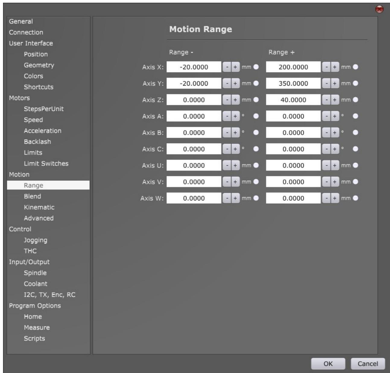
With *Range* values inserted, we set motion limits of machine. If we want machine to stop when limits are reached we must enable them. To enable Range limits for specified axis click the radio button:
