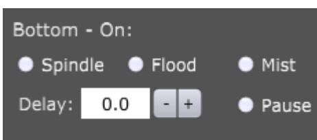
Inserts ON g-codes for Spindle, Flood, Mist (M3,M7,M8), Delay and Pause before cut, after moving down from Safe Height to cut (or pass) height.
